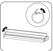
Open the cover on the top of the unit, and unclamp the bottom clamp on the cassette.
