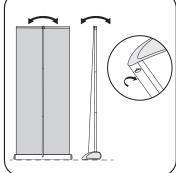
Adjust the threaded feet concealed underneath the base to level the unit if required.
