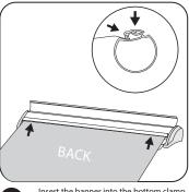
Insert the banner into the bottom clamp. The back of the banner should be facing upwards. Push the clamp fully shut. Gripping the banner close the cover.
