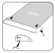
Ensure you are holding on tightly to the banner, then remove the pin found in the right side of the base and allow the banner to begin retracting into the base. Store the pin in the end cap.
