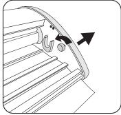
Remove the screw holding the left and right end caps, and remove them.
