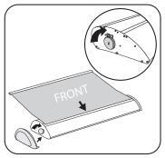
Rotate the graphic tensioner to finish retracting the banner into the base until it is fully retracted. When fully retracted, turn the graphic tensioner an additional two full turns to give the spring some extra strength. Place the end caps back onto the banner stand.
