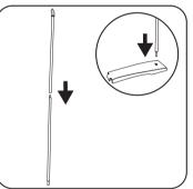
Assemble the support pole and place the bottom in the holder on the base.
