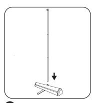
Assemble pole and insert the bottom of the pole in the center of the base.
