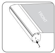
Gripping the banner securely with one hand, remove the locking pin from the right side of the base. Store the locking pin under the stand.
