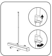
If the pole is telescopic, raise pole by opening latch, and secure at desired height.
