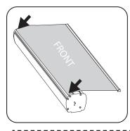
9 Carefully allow the banner to retract into the base, keeping it even distance from the edge of the base on both sides.
