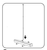
Assemble pole and insert the bottom of the pole in the center of the base. Ensure the pole is fully inserted onto the plastic fitting at the bottom of the base.
