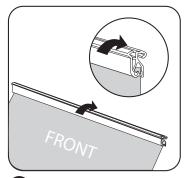
Press down firmly on clamp top bar to secure graphic into
