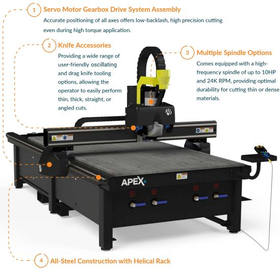
Engineered for high precision, every welded stress relieved steel frame is milled for both helical rack and rail allowing for smooth, uniform motion even in high torque applications.
