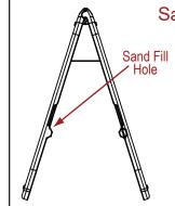
Each sign frame has two fill holes, one on each side of the frame.
