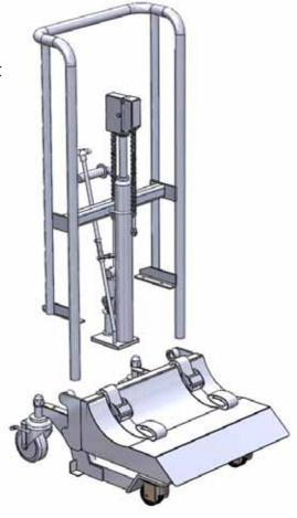
3. On the bottom of the hydraulic cylinder, line up the hole so that it rests on top of the boss on the caster frame.
