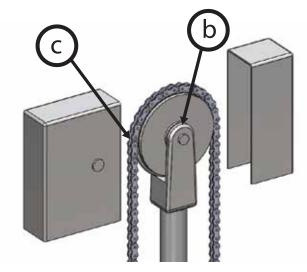
Remove screw to access the chain guide.
