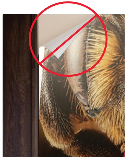
Not testing could result in a graphic that fails to adhere properly.
